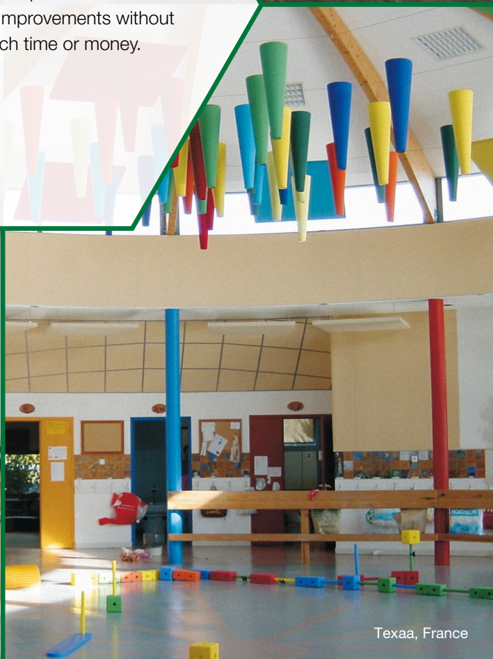
Baffles made of Basotect® in a school building | Merford, Netherlands
