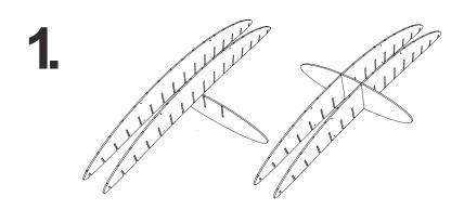
Sort the Lattice 'fins' into pairs, then into size order: largest to smallest. Start by taking one of the largest fins and slotting it into the centre slots in the 'rails'.
