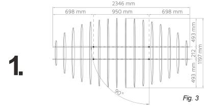
Determine where you want the Lattice to hang (Fig. 3). Mark the ceiling mount points as per the dotted lines.
