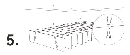
Lift the Lattice up to meet the cables and thread the wires through the plugs and into the cable adjuster.
