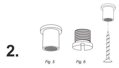
Separate the ceiling mounts into their individual parts - ceiling mounts (Fig. 5) and ceiling mount caps (Fig. 6).
