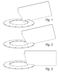
Start clipping the fins into the top ring as shown in Fig. 1, 2 and 3 until complete.
