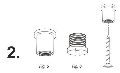
Separate the ceiling mounts into their individual parts - ceiling mounts (Fig. 5) and ceiling mount caps (Fig. 6).
