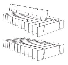
Once all the fins are inserted into the rail, flip the Lattice over 180°. Slide the remaining rail into the slots on the fins; again ensuring the tabs on the fins click into the groove on the rail.
