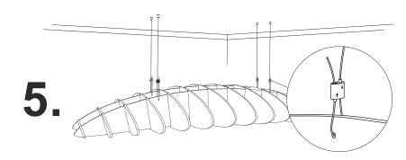
Lift the Lattice up to meet the cables threading the wires through the plugs and into the cable adjuster.
