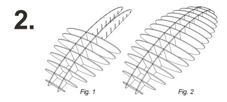
Finish one side by methodically inserting one of each pair into place in order of decreasing size (Fig. 1).
