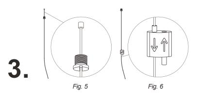
Thread the ceiling mount caps (Fig. 4) onto the cables (Fig. 5).
