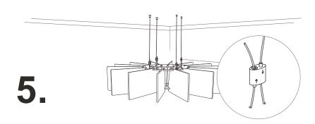
Lift the Lattice up to meet the cables, thread the wires through the holes in the top ring and insert into the cable adjuster.
