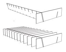
Lay one rail on its edge with the long slots facing up and methodically slot the fins into each slot on the rail at 90 degrees. Make sure the tabs on the fins click into the groove on the bottom of the rail.
