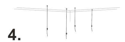
Screw assembled cables into the fixed ceiling mounts.
