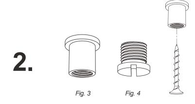
Separate the ceiling mounts into their individual parts - ceiling mounts (Fig. 3) and ceiling mount caps (Fig. 4).
