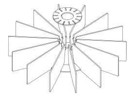
Once all fins are clipped to the top ring, gently and evenly press the bottom ring into position. Ensure all joints are snug and carefully roll over so the larger ring is on the top. Check again for any loose connections, make sure the hooks on the fins have clipped over the top ring.
