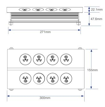
\*Corners of cut-outs must not be radiused. Suitable for table tops 10mm-30mm thick, and secured by the supplied 4x screw clamps.
